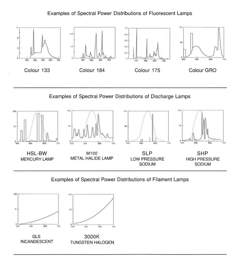
Fig 3 - Various spectral power distribution diagrams of common light sources
