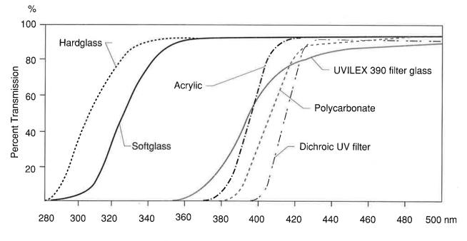
Fig 2 - Transmission values for various materials.
