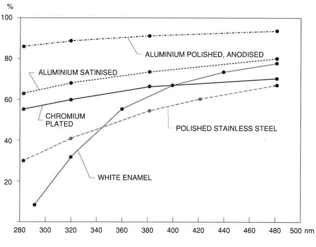
Fig 1 - Reflectance values for various materials in the visible (blue) and ultraviolet
